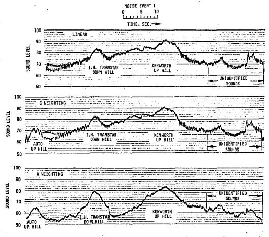
.Figure 3 - LEVEL RECORDINGS OF VEHICLE PASS-BY NOISE: NOISE EVENT 1 (Reference 3)
