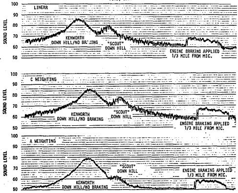
Figure 4 - LEVEL RECORDINGS OF VEHICLE PASS-BY NOISE: NOISE EVENT 2 (Reference 3)
