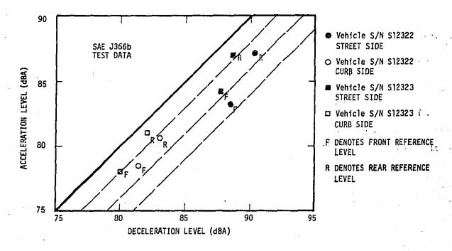
Figure 2 - ACCELERATION MODE SOUND LEVELS VERSUS DECELERATION MODE (WITH ENGINE BRAKE) SOUND LEVELS (SAEJ366b TESTS) FOR INTERCITY BUSES
